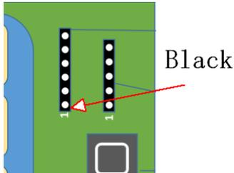
Use FTDR adapter TTL-232R-3V3 with 3.3V level from <http://www.ftdichip.com/Products/Cables/USBTTLSerial.htm>
